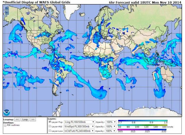
Figure 2 Example of WAFS gridded forecast for icing.
