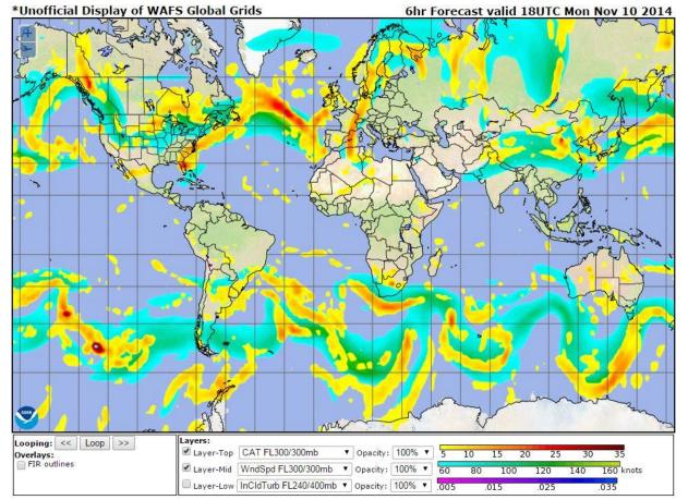
Figure 1 Example of WAFS gridded forecast for clear air turbulence and jet stream locations
